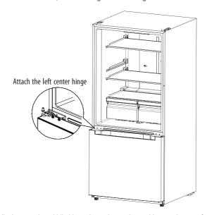
7)Put the refrigerator door vertically down on the middle hinge, then take out the top hinge and cover of other side from accessory bag, assemble top hinge, hinge cover and hole cover.
