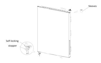
6)Remove the center hinge, then remove the center hinge shaft with a slotted screwdriver. Install the hinge shaft on opposite side of the hinge and install the hinge to the left of the box.
