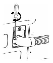
D. Fasten the drain hose to the two hose clamps on the washer frame with a Phillips screwdriver.
