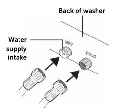
**CAUTION:** The water supply hose connected to the hot faucet must be connected to the hot water supply intake and the water hose connected to the cold faucet must be connected to the cold water supply intake.
