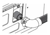
C. Secure the clamp with a flathead screwdriver (rotate clockwise) until it is tightly fitted.
