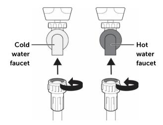
3. Tighten the fittings by hand until they are snug, and then tighten them an additional two-thirds of a turn with a wrench.
