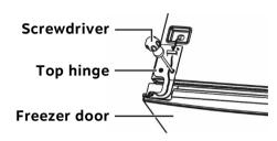
B. Install the top hinge cover from your spare parts bag with screws and a Phillips screwdriver, then reinstall the hole cover you removed previously on the other side.
