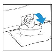
Place a towel and shallow container under the pump access door to protect the floor. It is normal for up to a quart of water to drain from
