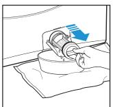
Turn the pump filter counterclockwise, and then pull out slowly to let the water drain.
