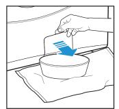
Open the access door by inserting a coin or screwdriver into the door notch, and then pull down the pour spout.
